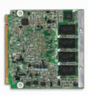
PQ7-M107 could be implemented in manufactory, transportation and automation applications. Better graphics performace, higher memory bandwidth are improved compared to BayTrail. In addition, HD Camera with MIPI CSI 2.0, 4k x 2k resolution and three independent displays are designed on PQ7-M107.
