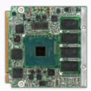
PQ7-M107 based on Qseven 2.0 SPEC designed with Intel® Atom™ N3000 series processor. Up to 4GB, 24bit LVDS, DP, USB 3.0
