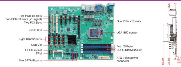
RUBY-D716VG2AR is based on Intel® Q87 chipset and desktop processor sku like Core™ i7 and i5. Build with PCI and PCI Express expensions, it is suitable for Medical, Industrial automation, and digital signage
